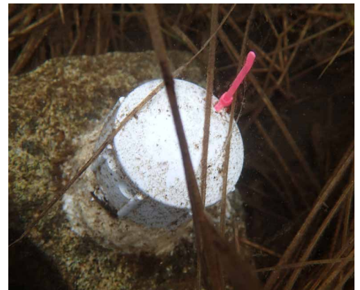
PVC pipe protects under-water data logger, which collects temperature data every 90 minutes. (Photo: Michael Lucid)
