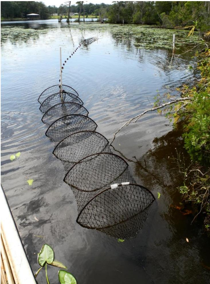
Figure 2. Paired hoop nets with interconnecting lead net (trammel). Funnel openings of the hoop nets face one another with the lead net acting as an aquatic drift fence directing active turtles into one of the hoop nets. No bait is needed with this trap configuration but may be used if desired.
