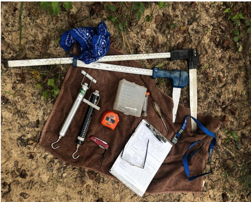
Figure 5. Equipment used to collect weights, measurements, and marking of Alligator Snapping Turtles. Present in the photograph are small and large Haglof calipers, a 5 m metric tape graduated in cm, 10 and 50 kg Pesola scales, cinch strap to be used with Pesola scale, notebook with data sheet, screwdriver and screws for marking, and box of 2 ml vials with 95% ETOH for tissue samples.
